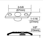
Optional bottom strike for fire openings using saddle thresholds or for flush floor mount. Must use for fire openings with 1/2" thresholds. Supplied with #10-24 x 1/2" machine screws and floor anchors.
