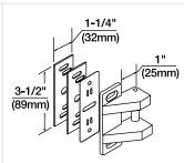
Optional strike for double door applications without a mullion. Supplied with #10-24 x 3/4" machine screws, two shims (each 1/16" thick), and one locking plate. Panic only.
