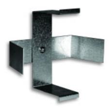
The **VE-RMB** attaches to the junction box supplied with Viking doorboxes and allows installation into existing walls. The bracket is screwed to the back of the junction box and provides a means of mounting even when no wall stud or support beam is accessible.
