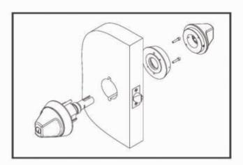
All locks provided are non-handed and 3 hour UL fire listed. The latch and dead latch are sintered stainless steel. The lock chassis is heavy duty wrought steel construction. Springs are tensioned for knob use and provide long life and smooth operation. Knobs are of stainless steel construction. Locks meet all requirements for ANSI grade 1 series 4000 locks. Locks fit into a standard ANSI 161 door preparation. 32D Finish. Schlage C keyway, standard
