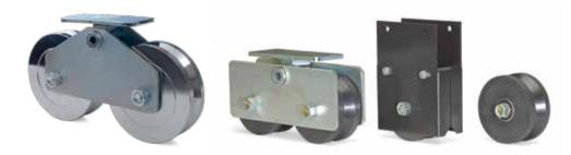
Available in sleeve and sealed roller bearings. Four inch and 6 inch sizes of either machined steel or UHMW. Maximum gate weights of up to 5000 lbs. V-Wheel assemblies include mounting bracket for 2x2 bottom rail. Tandem assemblies include pivoting mounting bracket. Tandem wheel assemblies provide superior performance for heavy gates by distributing the gate weight across 4 wheels instead of 2.
