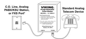
\* An FXS port lets you connect an analog telephone or device to an IP network.
