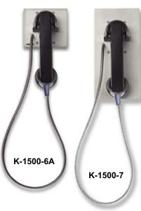
The K-1500 Series provides simple vandal resistant, communication in a flush mount, stainless steel, panel telephone. The K-1500-7 and K-1500-6A work ideally with Viking's DLE-200B line simulator or on a dedicated ringdown circuit. If dialing is necessary, use Viking's K-1900-7 or combine the K-1500 Series phones with Viking's K-1900-5 Hot-Line Dialer.
