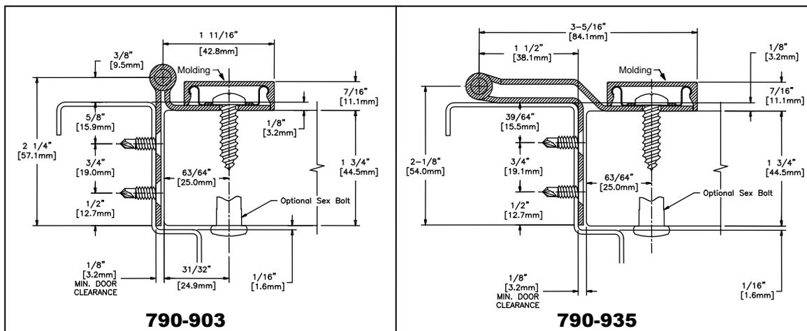
HAGER Models 790-903 and 790-935 are Stainless Steel Continuous Half Surface Hinges for 1-3/4" (44.5mm) thick doors. Clearance required between the hinge edge of the door and the frame rabbet is 1/8" (3.2mm) minimum. Both models provide for a 1/8" door inset. Model 790-935 provides 'swing clear' rotation.
