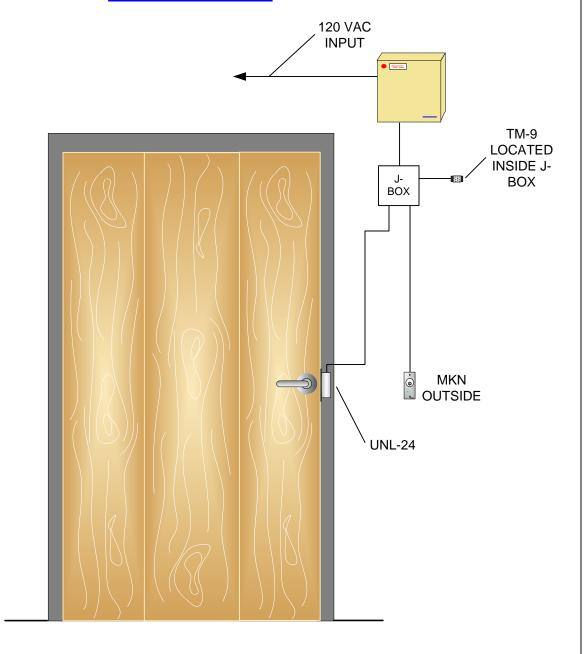
COMMENTS: MOST DEVICES COME WITH WIRE LEADS IN DIFFERENT LENGTHS DEPENDING ON WHAT MODEL IT IS. IF LONGER WIRE RUNS ARE REQUIRED 18G STRANDED WIRE IS FINE FOR SHORTER WIRE RUNS ON A 12 V SYSTEM. 22G WIRE IS ACCEPTABLE FOR SHORTER WIRE RUNS ON A 24 V SYSTEM. FOR SPECIFIC WIRE GUAGE QUESTIONS ON LONGER RUNS OR SYSTEMS PLEASE CALL OUR TECH SUPPORT LINE AT 1-800-MAGLOCK OR 1-800-624-5625.
