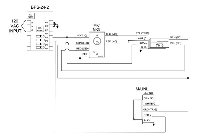
COMMENTS: MOST DEVICES COME WITH WIRE LEADS IN DIFFERENT LENGTHS DEPENDING ON WHAT MODEL IT IS. IF LONGER WIRE RUNS ARE REQUIRED 18G STRANDED WIRE IS FINE FOR SHORTER WIRE RUNS ON A 12 V SYSTEM. 22G WIRE IS ACCEPTABLE FOR SHORTER WIRE RUNS ON A 24 V SYSTEM. FOR SPECIFIC WIRE GUAGE QUESTIONS ON LONGER RUNS OR SYSTEMS PLEASE CALL OUR TECH SUPPORT LINE AT 1-800-MAGLOCK OR 1-800-624-5625.
