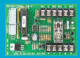
The TM-2 is a premium, industrial duty, multi-function timer that provides precise timing using stackable increments in seconds or minutes and easy-to-use dip switch settings.
