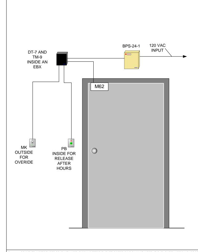
Comments: COMMENTS: MOST DEVICES COME WITH WIRE LEADS IN DIFFERENT LENGTHS DEPENDING ON WHAT MODEL IT IS. IF LONGER WIRE RUNS ARE REQUIRED 18G STRANDED WIRE IS FINE FOR SHORTER WIRE RUNS ON A 12 V SYSTEM. 22G WIRE IS ACCEPTABLE FOR SHORTER WIRE RUNS ON A 24 V SYSTEM. FOR SPECIFIC WIRE GUAGE QUESTIONS ON LONGER RUNS OR SYSTEMS PLEASE CALL OUR TECH SUPPORT LINE AT 1-800-MAGLOCK OR 1-800-624-5625.
