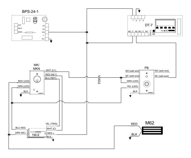
ADDITIONAL COMMENTS: Pushing the PB3ER unlocks UNL-24 on Restroom Door. Once inside the occupant pushes the PB4 to lock out the trigger to the UNL-24 by latching the RLP-24. When the door is opened by the occupant the lock status changes state and resets the RLP-24. The Mortise Key switch, MK, is available to override the lock (should someone pass out, etc. in the Restroom). Red LED indicates Restroom is Occupied and Green LED indicates that the Restroom is available.
