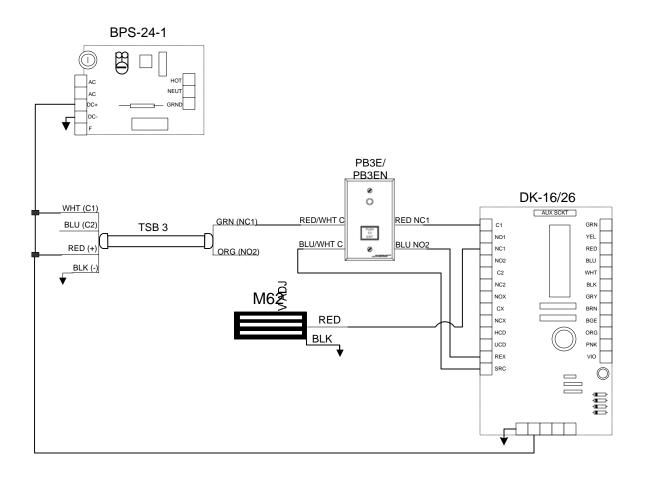
COMMENTS: MOST DEVICES COME WITH WIRE LEADS IN DIFFERENT LENGTHS DEPENDING ON WHAT MODEL IT IS. IF LONGER WIRE RUNS ARE REQUIRED 18G STRANDED WIRE IS FINE FOR SHORTER WIRE RUNS ON A 12 V SYSTEM. 22G WIRE IS ACCEPTABLE FOR SHORTER WIRE RUNS ON A 24 V SYSTEM. FOR SPECIFIC WIRE GUAGE QUESTIONS ON LONGER RUNS OR SYSTEMS PLEASE CALL OUR TECH SUPPORT LINE AT 1-800-MAGLOCK OR 1-800-624-5625.
