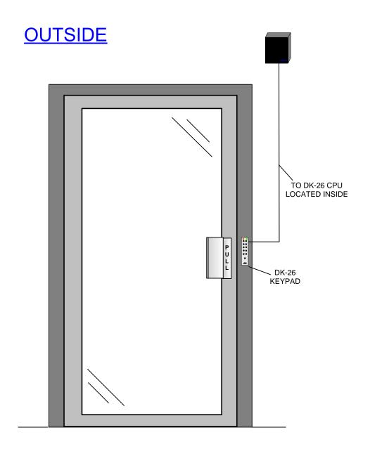
COMMENTS: MOST DEVICES COME WITH WIRE LEADS IN DIFFERENT LENGTHS DEPENDING ON WHAT MODEL IT IS. IF LONGER WIRE RUNS ARE REQUIRED 18G STRANDED WIRE IS FINE FOR SHORTER WIRE RUNS ON A 12 V SYSTEM. 22G WIRE IS ACCEPTABLE FOR SHORTER WIRE RUNS ON A 24 V SYSTEM. FOR SPECIFIC WIRE GUAGE QUESTIONS ON LONGER RUNS OR SYSTEMS PLEASE CALL OUR TECH SUPPORT LINE AT 1-800-MAGLOCK OR 1-800-624-5625.
