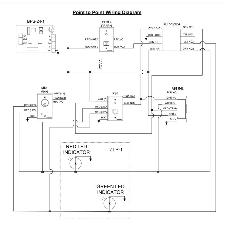
ADDITIONAL COMMENTS: Pushing the PB3ER unlocks UNL-24 on Restroom Door. Once inside the occupant pushes the PB4 to lock out the trigger to the UNL-24 by latching the RLP-24. When the door is opened by the occupant the lock status changes state and resets the RLP-24. The Mortise Key switch, MK, is available to override the lock (should someone pass out, etc. in the Restroom). Red LED indicates Restroom is Occupied and Green LED indicates that the Restroom is available.
