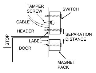
door. The magnet pack should then be mounted as shown. Drill 7/64" (2.75MM) diameter pilot holes for the #8 mounting screws.
