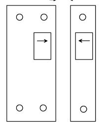
THE ARROWS ON THE SWITCH AND MAGNET PACK MUST FACE EACH OTHER AND AND THE ENDS OF EACH COMPONENT MUST BE EVEN- NOT OFFSET.
