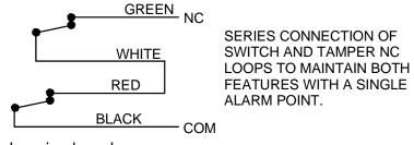
the switch module is tampered with while the door is closed.
