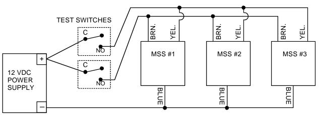
REMOTE TEST WIRING SHOWN WITH THREE MSS SWITCHES. ANY NUMBER OF MSS SWITCHES CAN BE CONNECTED IN THIS WAY. NOTE THE TWO NORMALLY OPEN TEST SWITCHES. THEY SHOULD BE CLOSED ONE AT A TIME AND ALL MSS SWITCHES SHOULD GO INTO ALARM TWICE TO PASS THE TEST.
