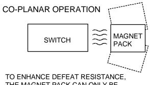
TO ENHANCE DEFEAT RESISTANCE, THE MAGNET PACK CAN ONLY BE READ IN A NARROW ANGLE IN FRONT OF THE SWITCH.
