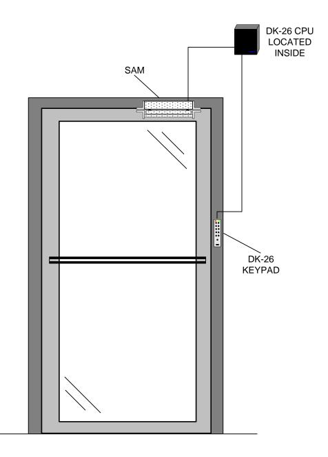
COMMENTS: MOST DEVICES COME WITH WIRE LEADS IN DIFFERENT LENGTHS DEPENDING ON WHAT MODEL IT IS. IF LONGER WIRE RUNS ARE REQUIRED 18G STRANDED WIRE IS FINE FOR SHORTER WIRE RUNS ON A 12 V SYSTEM. 22G WIRE IS ACCEPTABLE FOR SHORTER WIRE RUNS ON A 24 V SYSTEM. FOR SPECIFIC WIRE GUAGE QUESTIONS ON LONGER RUNS OR SYSTEMS PLEASE CALL OUR TECH SUPPORT LINE AT 1-800-MAGLOCK OR 1-800-624-5625.
