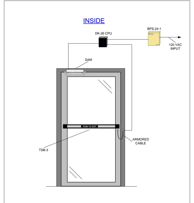
COMMENTS: MOST DEVICES COME WITH WIRE LEADS IN DIFFERENT LENGTHS DEPENDING ON WHAT MODEL IT IS. IF LONGER WIRE RUNS ARE REQUIRED 18G STRANDED WIRE IS FINE FOR SHORTER WIRE RUNS ON A 12 V SYSTEM. 22G WIRE IS ACCEPTABLE FOR SHORTER WIRE RUNS ON A 24 V SYSTEM. FOR SPECIFIC WIRE GUAGE QUESTIONS ON LONGER RUNS OR SYSTEMS PLEASE CALL OUR TECH SUPPORT LINE AT 1-800-MAGLOCK OR 1-800-624-5625.
