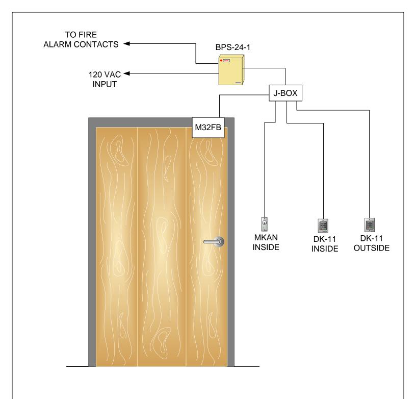
COMMENTS: MOST DEVICES COME WITH WIRE LEADS IN DIFFERENT LENGTHS DEPENDING ON WHAT MODEL IT IS. IF LONGER WIRE RUNS ARE REQUIRED 18G STRANDED WIRE IS FINE FOR SHORTER WIRE RUNS ON A 12 V SYSTEM. 22G WIRE IS ACCEPTABLE FOR SHORTER WIRE RUNS ON A 24 V SYSTEM. FOR SPECIFIC WIRE GUAGE QUESTIONS ON LONGER RUNS OR SYSTEMS PLEASE CALL OUR TECH SUPPORT LINE AT 1-800-MAGLOCK OR 1-800-624-5625.
