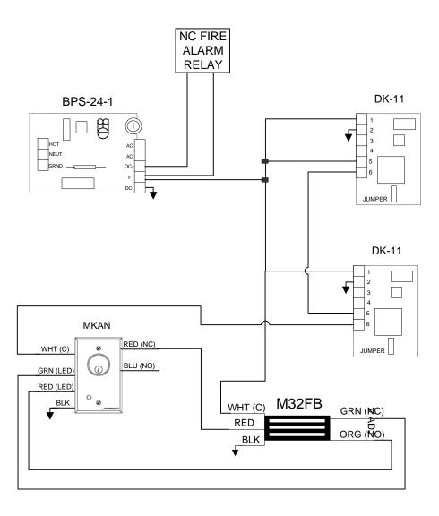
COMMENTS: MOST DEVICES COME WITH WIRE LEADS IN DIFFERENT LENGTHS DEPENDING ON WHAT MODEL IT IS. IF LONGER WIRE RUNS ARE REQUIRED 18G STRANDED WIRE IS FINE FOR SHORTER WIRE RUNS ON A 12 V SYSTEM. 22G WIRE IS ACCEPTABLE FOR SHORTER WIRE RUNS ON A 24 V SYSTEM. FOR SPECIFIC WIRE GUAGE QUESTIONS ON LONGER RUNS OR SYSTEMS PLEASE CALL OUR TECH SUPPORT LINE AT 1-800-MAGLOCK OR 1-800-624-5625.
