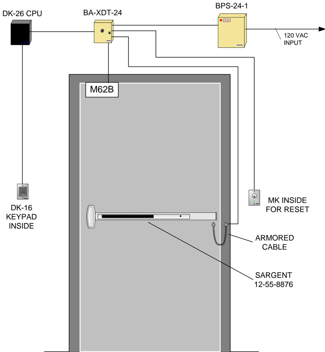
COMMENTS: MOST DEVICES COME WITH WIRE LEADS IN DIFFERENT LENGTHS DEPENDING ON WHAT MODEL IT IS. IF LONGER WIRE RUNS ARE REQUIRED 18G STRANDED WIRE IS FINE FOR SHORTER WIRE RUNS ON A 12 V SYSTEM. 22G WIRE IS ACCEPTABLE FOR SHORTER WIRE RUNS ON A 24 V SYSTEM. FOR SPECIFIC WIRE GAUGE QUESTIONS ON LONGER RUNS OR SYSTEMS PLEASE CALL OUR TECH SUPPORT LINE AT 1-800-MAGLOCK OR 1-800-624-5625.
