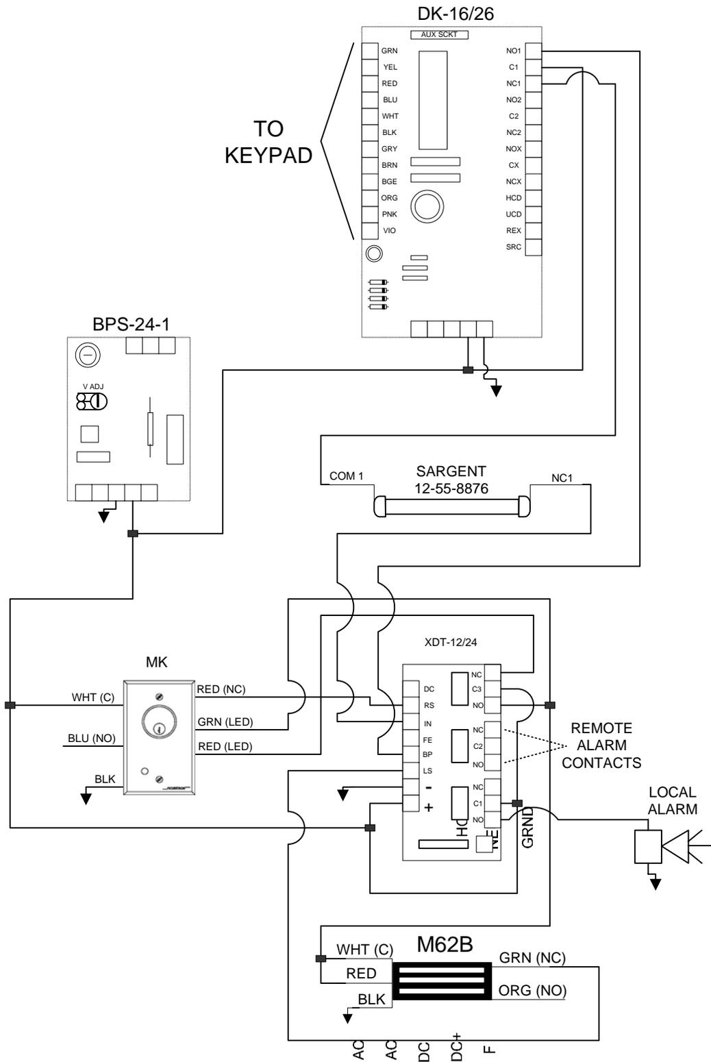
COMMENTS: MOST DEVICES COME WITH WIRE LEADS IN DIFFERENT LENGTHS DEPENDING ON WHAT MODEL IT IS. IF LONGER WIRE RUNS ARE REQUIRED 18G STRANDED WIRE IS FINE FOR SHORTER WIRE RUNS ON A 12 V SYSTEM. 22G WIRE IS ACCEPTABLE FOR SHORTER WIRE RUNS ON A 24 V SYSTEM. FOR SPECIFIC WIRE GAUGE QUESTIONS ON LONGER RUNS OR SYSTEMS PLEASE CALL OUR TECH SUPPORT LINE AT 1-800-MAGLOCK OR 1-800-624-5625.
