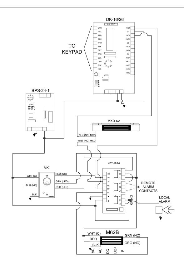
COMMENTS: MOST DEVICES COME WITH WIRE LEADS IN DIFFERENT LENGTHS DEPENDING ON WHAT MODEL IT IS. IF LONGER WIRE RUNS ARE REQUIRED 18G STRANDED WIRE IS FINE FOR SHORTER WIRE RUNS ON A 12 V SYSTEM. 22G WIRE IS ACCEPTABLE FOR SHORTER WIRE RUNS ON A 24 V SYSTEM. FOR SPECIFIC WIRE GUAGE QUESTIONS ON LONGER RUNS OR SYSTEMS PLEASE CALL OUR TECH SUPPORT LINE AT 1-800-MAGLOCK OR 1-800-624-5625.
