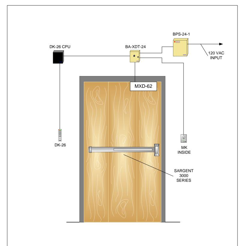
COMMENTS: MOST DEVICES COME WITH WIRE LEADS IN DIFFERENT LENGTHS DEPENDING ON WHAT MODEL IT IS. IF LONGER WIRE RUNS ARE REQUIRED 18G STRANDED WIRE IS FINE FOR SHORTER WIRE RUNS ON A 12 V SYSTEM. 22G WIRE IS ACCEPTABLE FOR SHORTER WIRE RUNS ON A 24 V SYSTEM. FOR SPECIFIC WIRE GUAGE QUESTIONS ON LONGER RUNS OR SYSTEMS PLEASE CALL OUR TECH SUPPORT LINE AT 1-800-MAGLOCK OR 1-800-624-5625.
