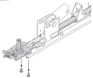
2. Drill or use center punch on two rivet heads until rivets can be removed from baseplate.
