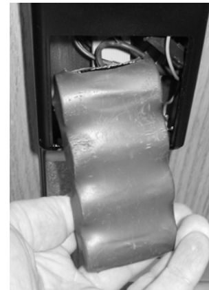
FIG. D: INSERT BATTERY PACK INTO HOUSING ("SEALED" TYPE SHOWN)
