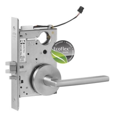
The Corbin Russwin ML20900 ECL Electromechanical Lock, is an ANSI/BHMA A156.13 Series 1000 Grade 1 mechanical mortise lock. It has a reversible latch with stainless steel insert and an independent non-handed stainless steel deadlatch.
