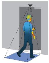
Reduces False Detections by Detecting Both Presence and a Change in Temperature
