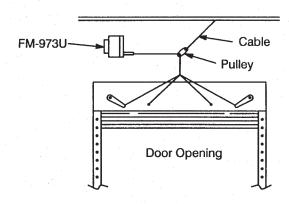
Figure 1. Rolling steel fire door shown above. The FM-973U is adaptable to many other doors or shutters through the use of various linkage systems.
