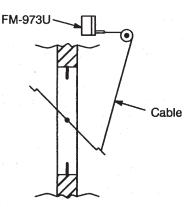
**Figure 3.** Center pivoted self-closing window.
