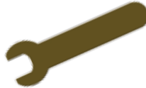
EHW Extension Wrenches Used to tighten extension rods to catch plate assembly
