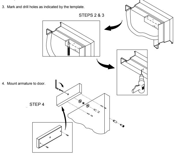
Install mounting plate to header with the interlock detail away from the door side of the stop. Loosely fasten screws through adjustment slot as shown. Assure that the mounting plate and armature line up properly, then tighten down <u>ALL</u> mounting screws.
