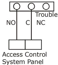
The diagram shows basic wiring to provide output to a control panel or local alarm for notification of over-voltage or under-voltage.
