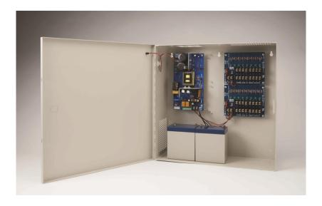
6 Amp Dual Voltage Power Supply: converts 115VAC or 240VAC into 12 or 24VDC with over 90% efficiency, metal enclosure protects from tamper and accidental contact.
