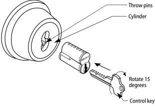
Figure 10 — Installing the core
