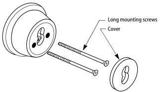
Figure 8 — Installing the inside cylinder mounting screws & cover
