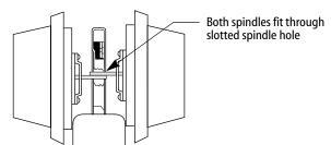
Figure 7 — Side view of double-keyed cylinder deadbolt spindles
