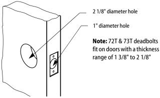
Figure 2 — Boring two holes
