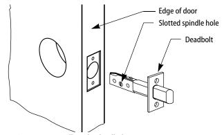
Figure 5 — Installing the deadbolt
