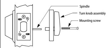
Figure 9 — Installing the inside trim
