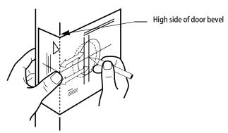
Figure 1 — Marking the template
