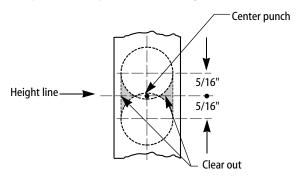
Figure 3 — Drilling out the deadbolt recess
