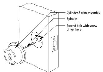
Figure 6 — Installing the cylinder
