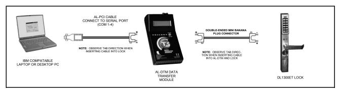
Scenario 2 Create the program in DL-Windows and transfer the program from your computer to an AL-DTM (via an AL-PCI cable)... then transfer the program from the AL-DTM to the lock(s) (via a double-ended mini banana plug). The hand-held AL-DTM is useful because you do not have to transport (or find electricity for) your computer. Data can also flow in reverse, from the lock, through the AL-DTM, back to the computer for examination.
