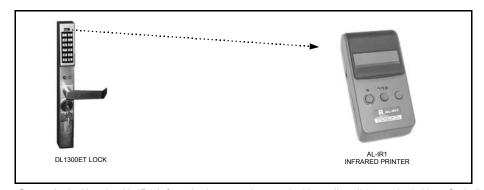
Scenario 3 Use the AL-IR1 Infrared printer to print your lock's audit trail (event log), User Code list, clock settings and software version. No cable required.
