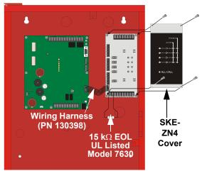
Figure 3: View With SKE-ZN4 Installed
