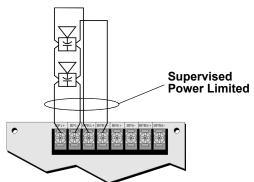
Figure 6: Class A (Style Z) Speaker Configuration
