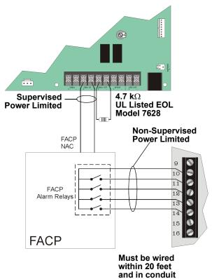
Figure 7: FACP Alarm Control Outputs
