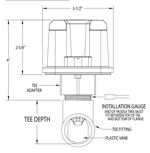
DESIGNED TO FIT WITHIN 2 X 4 STUD WALL CONSTRUCTION
