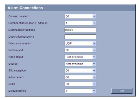
You can select how the VIP X1600 XFMD responds to an alarm. In the event of an alarm, the unit can automatically connect to a pre-defined IP address. You can enter up to ten IP addresses to which the VIP X1600 XFMD will connect in sequence in the event of an alarm, until a connection is made.
