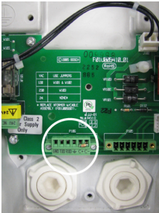
Figure 4.1: P106 connector with 100 Ohm resistor
