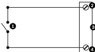
**Figure 4.3** N.O. - Normally Open Non-supervised Connections
