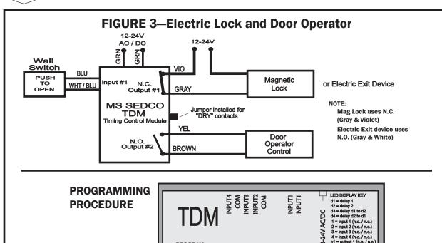
Once the TDM has been wired for the above application, programming of the device is as follows:
