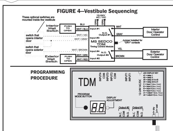
Once the TDM has been wired for the above application, programming of the device is as follows:
