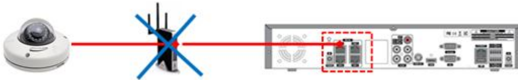
Figure 2.5.2. Incorrect connection with the PoE Ports
