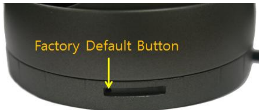
Figure 2-6 Factory Default switch of OIPC22T7G
