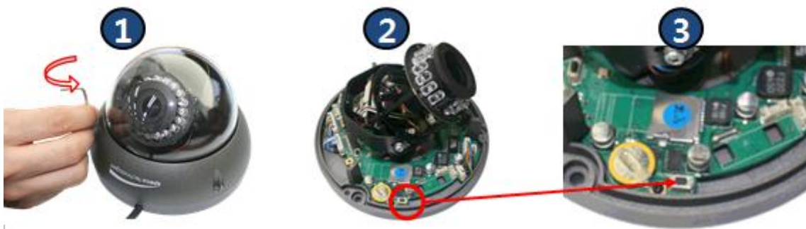
Figure 2-5. Factory Default Switch of ONSIP O2D4
