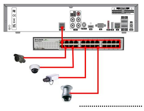
Figure 2.6.1.1. Proper connection example of the NS (No PoE Switch).
