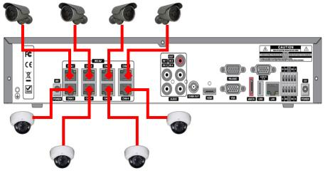
Figure 2.5.1.1 IP Camera Connection Diagram (N8NSP)
