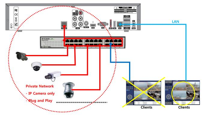
Figure 2.6.1.2. Improper connection of the NS (No PoE switch).
