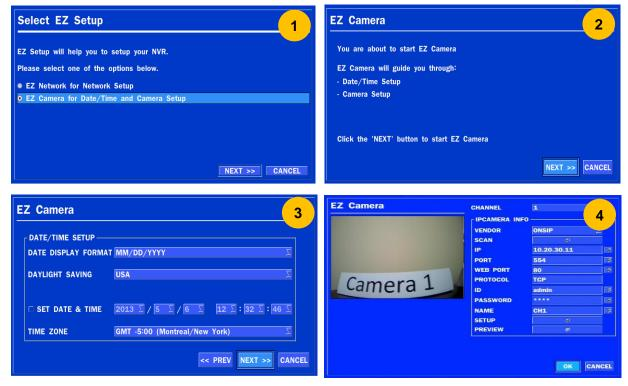
Figure 2.4.1. EZ CAMERA Setup Procedure
