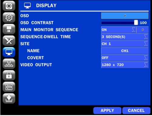
Figure 4.5.1. DISPLAY Setup Screen
