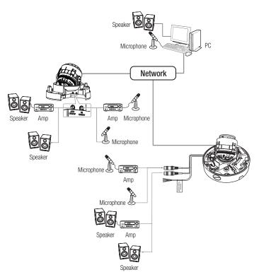
Connect the AUDIO IN port of the camera with the microphone or LINE OUT port of the amplifier that the microphone is connected to.
