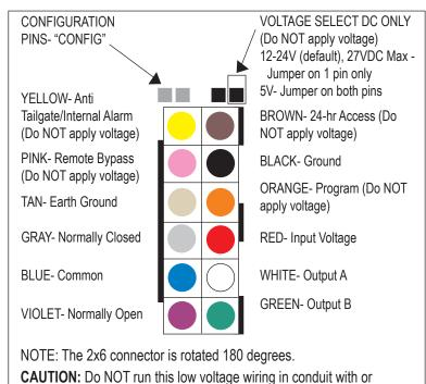
adjacent to line voltage wiring.
