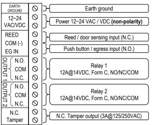
Earth ground terminal: Connect a <u>continuous wire</u> from the Earth Ground terminal to a grounding point to avoid damage from static discharge. If using an AC adapter for power input, do not connect the AC adapter output to Earth Ground.
