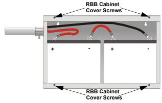
Figure 3: Battery Connections in the RBB Cabinet
