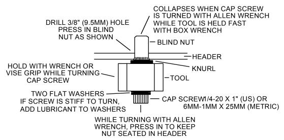
FIG. 5: TYPICAL MOUNTING ON OUTSWINGING DOOR
