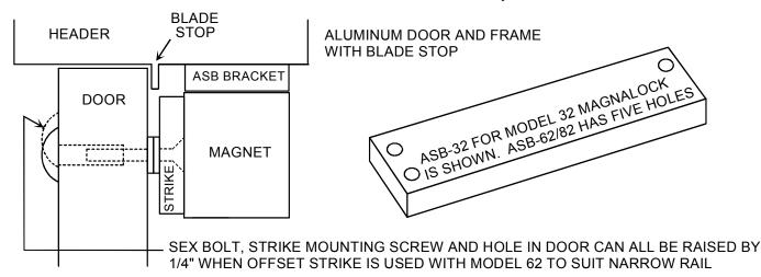
Note: When using the ASB on Aluminum Frame Glass Doors with the M82SC or M62 the strike mounting hardware may need to be installed too close to the glass for this reason it is recommend that the **Offset Strike** option be used M62-OS or M82SC-OS.
