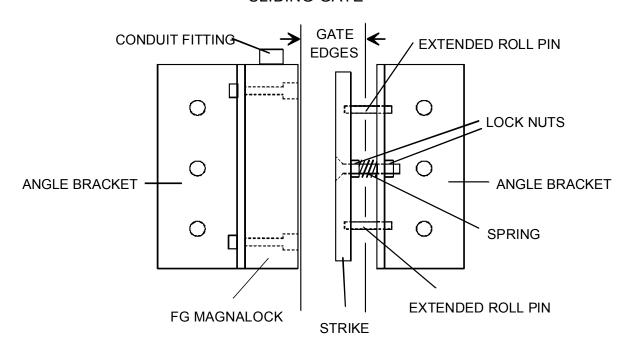
The drawings in figure 12 describe three typical gate applications single swing gates, double swing gates and sliding gates. The strike plate cannot be welded to the gate it must be
