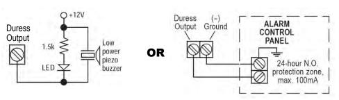
When a duress code is entered, the duress output will switch to (-) ground. It can trigger a connected LED lamp or small buzzer to notify a guard, or connect it to a 24 hour N.O. alarm system protection zone.
