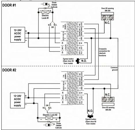
Mantrap (Interlock) - Each keypad can be used as a stand-alone keypad. The mantrap feature is for a protected area with two doors to ensure only one door can be opened at a time. With the mantrap feature enabled, when a user opens one door either by entering a code or with a requestto-exit button, a signal is sent to the second keypad to disable it, thereby preventing access through the second door until the first door is closed.
