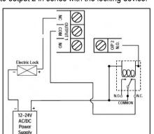
• For N.C. locking devices: Connect a relay • For N.O. locking devices: Connect a relay to output 2 in parallel with the locking device.
