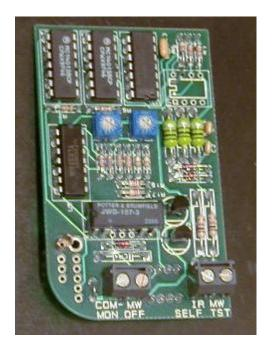
3. If RF SHUT-OFF or remote SELF-TEST is to be utilized with a different power source than the one powering the sensor, cut Jumper J1 and route DC voltage (both pos. and neg.) to SHUT-OFF and COMMON TERMINALS. (Note: This procedure is for ground-loop prevention).
