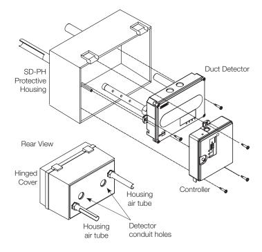
The SD-PH is easy to install and service. The hinged and transparent cover provides ready access to the detector, while keeping its status indicators visible at all times.
