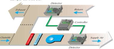
facing the airstream. Sampling tubes may be rotated in 45-degree increments so that air-holes can be aligned to allow the unit to be mounted in virtually any angle relative to the airflow.
