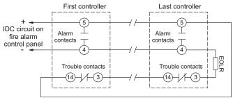
End-of-line resistor required on last device for circuit supervision. Use resistor value specified by the fire alarm panel manufacturer. Note: This configuration is not allowed when using remote test stations.
