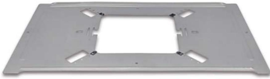
The **SA-TBA** is a tile bridge designed to mount 8 inch loud speaker and bridges both 2 ft x 2 ft and 2 ft x 4 ft ceiling tiles. It is compatible with the Viking models **SA-1S**, **30AE**, **35AE**, and **40AE** speakers. The **SA-TBA** tile bridge is constructed of 24 gauge cold rolled steel with an electro galvanized rust-resistant finish.
