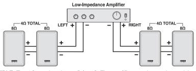
**EXAMPLE:** Two  $8\Omega$  speakers in parallel =  $4\Omega$ . The amplifier must be rated to work into  $4\Omega$  loads. Also in this example, the max amplifier output power rating (each channel into  $4\Omega$ ) should not exceed 150W for S4/T (2 X 75W) speakers or 300 for S5/T (2 X 150W).
