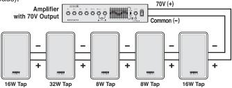
**EXAMPLE:** 16 + 32 + 8 + 8 + 16 = 80 Watts minimum amplifier output power rating.
