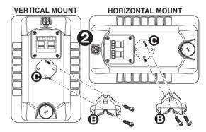
3. Connect the speaker wires to the rear input terminals on the loudspeaker. Set the speaker with Mounting Cup Bracket (B) over the Mounting Base (A). Loosely screw the Mounting Cap Nut (D) onto the Mounting Base threaded stud.
