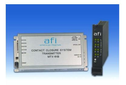
The American Fibertek 81B Series multiplexes 8 total channels (4 in each direction) of dry latching contact closure on one multimode fiber. A user selectable feature allows the contact status to be maintained unchanged or reset through power-cycle and loss-of-optical-power. A reset button is available to clear all contact status to the default state. Individual channel LEDs on the transmitter and the receiver units indicate the channel status.
