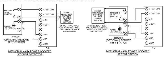
NOTE: THE USE OF THE RTS151 REQUIRES THE INSTALLATION OF AN ACCESSORY COIL, DCOIL, SOLD SEPARATELY.
