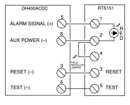
FIGURE 8. WIRING DIAGRAM FOR RTS151 TO BEAM1224/ BEAM1224S SMOKE DETECTOR:
